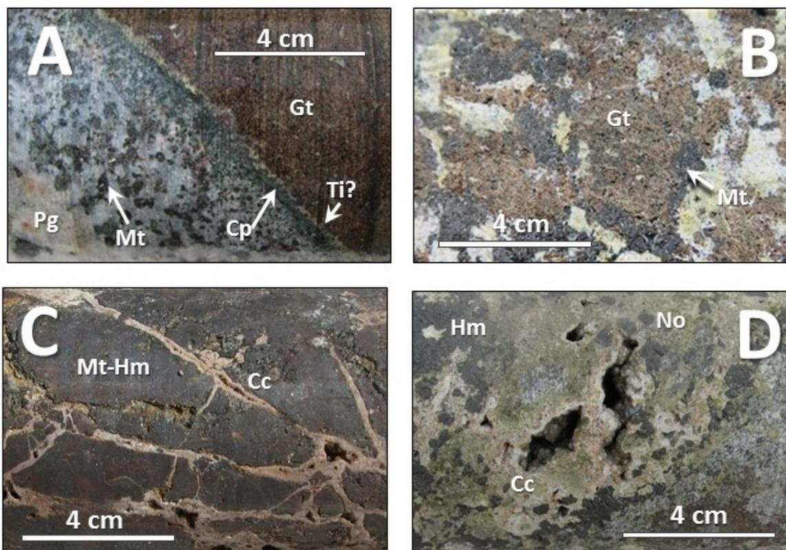
Figure 5. Images of outcrop and core from Inca. A - Contact between pegmatite (Pg, left) and garnetite (Gt, right). Magnetite (mt) is enriched at the contact zone and there is a thin rind of clinopyroxene (cp) and a possible Ti oxide (Ti?) right at the contact; B - Residual garnetite (gt) with magnetite (mt) rims; C - Massive magnetite-hematite rock cut by vuggy calcite-nontronite veins. D - Close-up of vuggy calcite-nontronite breccia cement.
