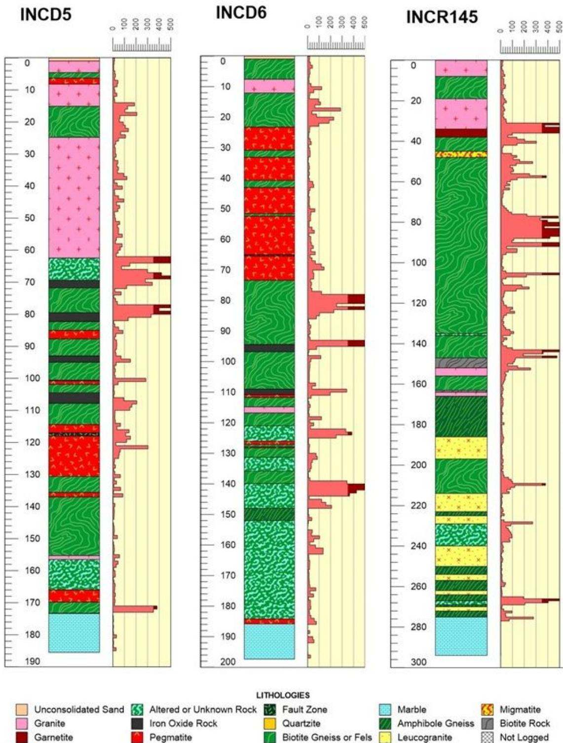
Figure 4. Representative strip logs of diamond drill holes from Inca. The histograms are uranium content as ppm  $U_3O_8$ . Garnetite, iron oxide rock and “altered or unknown rock” are varieties of skarn. Many other types of skarn rocks were not differentiated from the host, partly because amphibole- or pyroxene-rich skarn is patchily developed.
