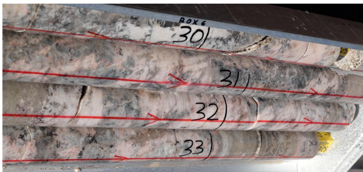
Figure 2. Petalite-bearing pegmatite in HQ drill core. Depths in metres
