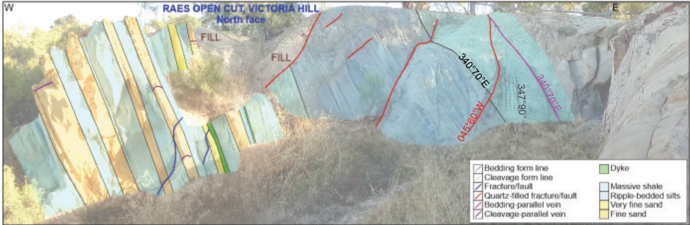
Site 8. Geology of part of the south side of Rae's open cut showing weakly developed limb thrust faults with very little offset and some quartz veining. Some mine fill on limb thrusts can be seen. The eastern side of the cutting is a thick shaley succession of ripple-bedded silts at the base grading to laminated and massive shale, the latter hosting a 10 cm laminated quartz vein.
